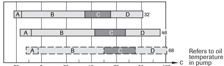
E.g. Hydraulic oil 32: The designation "32" denotes the viscosity is 32 cSt at 40 °C. Lowest start temperature is -23 °C and highest working temperature 82 °C. Ideal working temperature is 35 - 55 °C.
