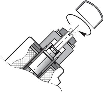
If it is necessary to run a hydraulic function as an emergency operation during a power cut, the pump flow can be started manually by screwing in the By-Pass valve setting screw.
