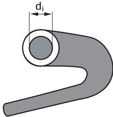
If the suction pipe is more than 2 m long the internal diameter must be increased by 10 mm for each meter extension.
