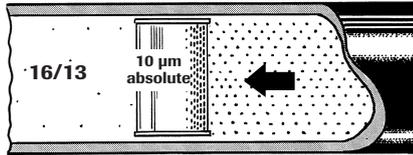
Max 64,000 particles  $> 5 \mu\text{m}/100 \text{ ml}$ .
